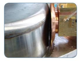
CEMSA manufacture automatic seam welding solutions, like the "ROBOSEAM", for high quality welding, in a cooling water bath, delicate materials sensible at the overheating (stainless steel in different grades), on a working table with a copper plate of variable sizes up to cm 1000 x 2000 mm
