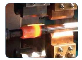
This technology enables the end user to carry on machining works just in the area where the deformation occurs, starting from a bar/tube of lower thickness and diameter, saving a great amount of material
