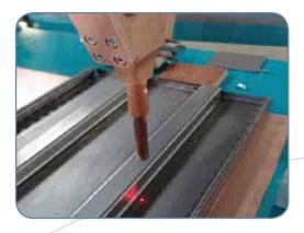
In the attached picture, it is possible to see a welding head of a "ROOF" model, the most flexible solution for assembly and manufacturing metallic doors and cabinets of any kind, available as well in its automatic version "ROBOSIDE".
