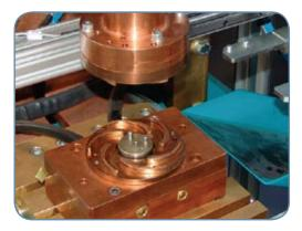
Specifically for welding automotive parts, additional controls in real time on pressure, heating and penetration become essential for certifying the quality of each output. Collecting these data for each cycle makes possible a constant monitoring of the production process.
