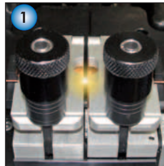
1 Join the end wire from drum 1 with the start wire from drum 2 using the Butt Welder.
