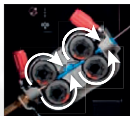
4 rolls/ all driven: • eliminates wire slipping • no wire deformation
