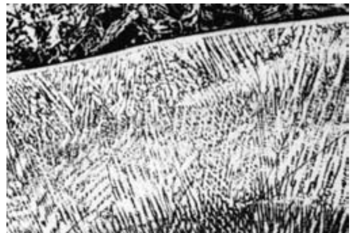
Fig. 8. Unalloyed sheet steel clad with ESAB OK 92.26. Fusion zone boundary is fault-free with no cracks. Mn content of weld metal is 5 %. (200x).
