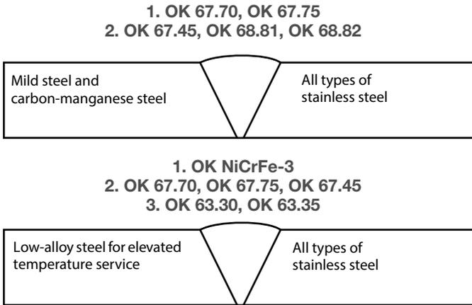
Never use unalloyed electrodes for these joints:
