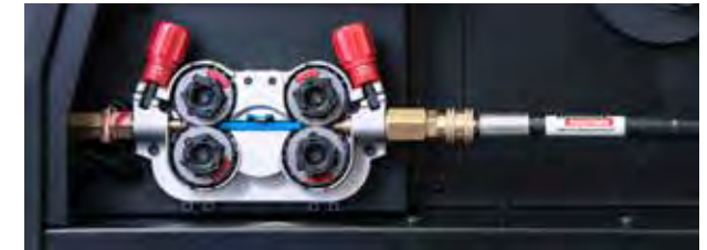
Connection for drum feed (optional adapter). Less need to change wire spools saves time
