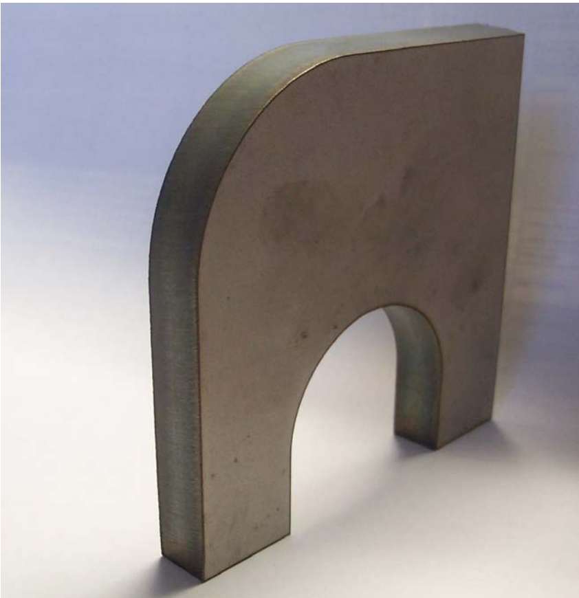
Subtitle: 12 mm Stainless Steel cutting sample WMS™ process. Vertical cut, oxide free and dress free.
