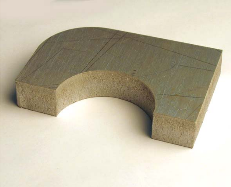
Subtitle: 20 mm Aluminium cutting sample using WMS™ process. We can notify the reduced rugosity on the cutted surface compared with normal Plasma cutting.
